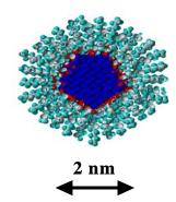
particle covered by a monolayer of ligand) was studied by TPR and TPD reactions. The particles sintered during treatment in  $H_2$  at 400 °C, while their size increases only slightly in inert atmosphere. The amount of grafted ligand could be quantified by analyzing the desorbing gases from the surface during heating.
